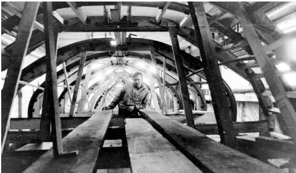
November 1978. Yura Bondar began building Gonta at the very end of July 1978. Though the yacht had no name then. So far only the moulds are standing. Ahead – three years of single-minded work!
